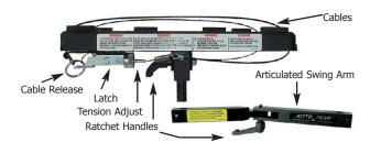
Model 5340ACD is an ergonomic, multi-adjustable swing arm desk used as a platform for mobile professionals to secure and comfortably use a notebook computer in a vehicle. The Cable-Dock® securing system utilizes two (2) nylon coated steel cables that wrap up and over the whole computer for a firm and positive grip. The "Original" articulated swing arm enables you to pull the desktop over for comfortable operation, reducing back strain.
