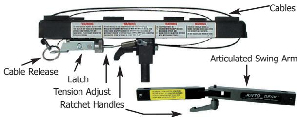
Model 5315ACD is an ergonomic, multi-adjustable swing arm desk used as a platform for mobile professionals to secure and comfortably use a notebook computer in a vehicle. This model will mount to all vehicles with top bolting passenger seat rails that are 12" to 17" apart. Inquire about our other No Holes Mounts that are available for vehicles with angled seat rails.
